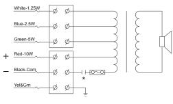
\* unit fitted with capacitor
